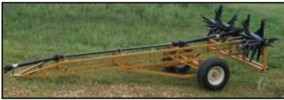
An example of a paddlewheel aerator
